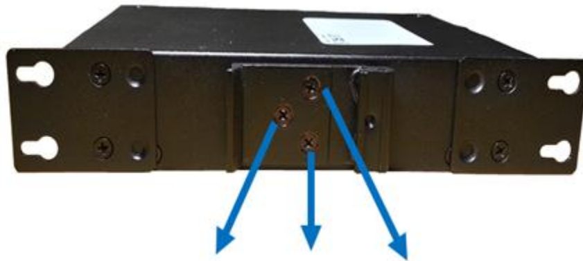
Figure 3.4 - Remove DIN-Rail bracket from the Switch
